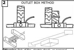
Warning-Risk of fire, electric shock, or personal injury. The fan in this box may be either directly supported from a structural framing member of a building and/or may be mounted to an outlet box marked acceptable for fan support of of 31.8 kg(70lbs) or less. Most outlet boxes commonly used for the support of lumminaires may not be acceptable for fan support and may need to be replaced. Consult a qualified electrician if in doubt
